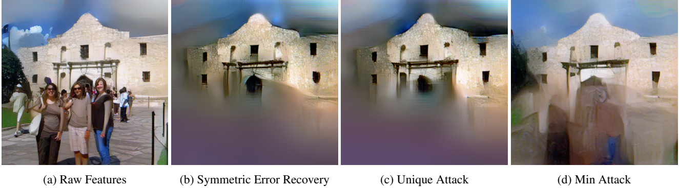
Figure 4: Inversion attacks for localization with private queries. Recovered image using: (a) the complete set of features, (b) points recovered from the proposed method which includes the symmetric check, (c) additional points recovered from inlier-outlier selecting points with unique matches, (d) taking the closest candidate.
